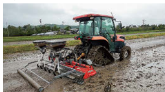
Sowing of uncoated paddy rice seeds using a submerged shallow soil seeder
