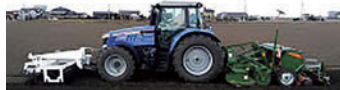
Combined work of plowing, soil crushing, and seeding in the direct sowing cultivation of paddy rice in dry fields
