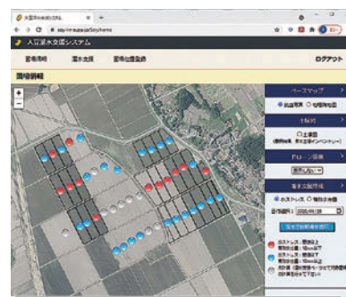
Soybean irrigation support system that can estimate drought damage in real-time (red circles indicate fields that require irrigation)
