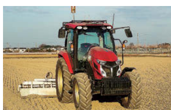
An unmanned labor-saving field leveler that enables high-speed and high-precision leveling using GNSS data and UAV acquisition images (left) and a harvester specific for grain corn (right) in the high-efficiency crop rotation system
