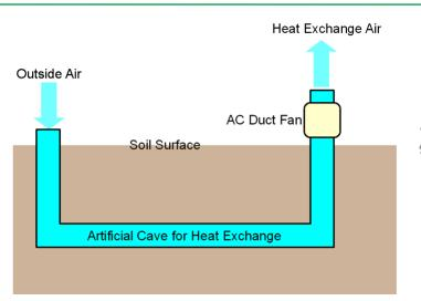
To obtain heat exchange air stably a AC duct fan was installed.
