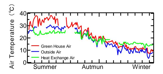
Underground heat exchange air showed the expected temperature. However, since its amount is too small to control the temperature of the entire greenhouse. Also because of the effect of wind, the flow rate was unstable.
