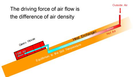
Schematic diagram of the underground heat exchanger
