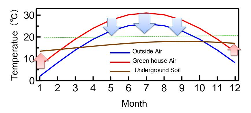
Soil temperature is almost constant throughout the year (deeper than a few meters). By achieving equilibrium to the soil temperature, we can obtain cooler air in summer and warmer air in winter which is suitable temperature for the crop.
