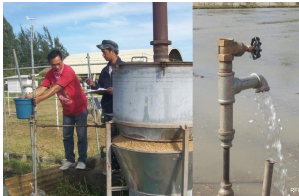
Figure 7. The carbonizer-water pump undergoing field test.
