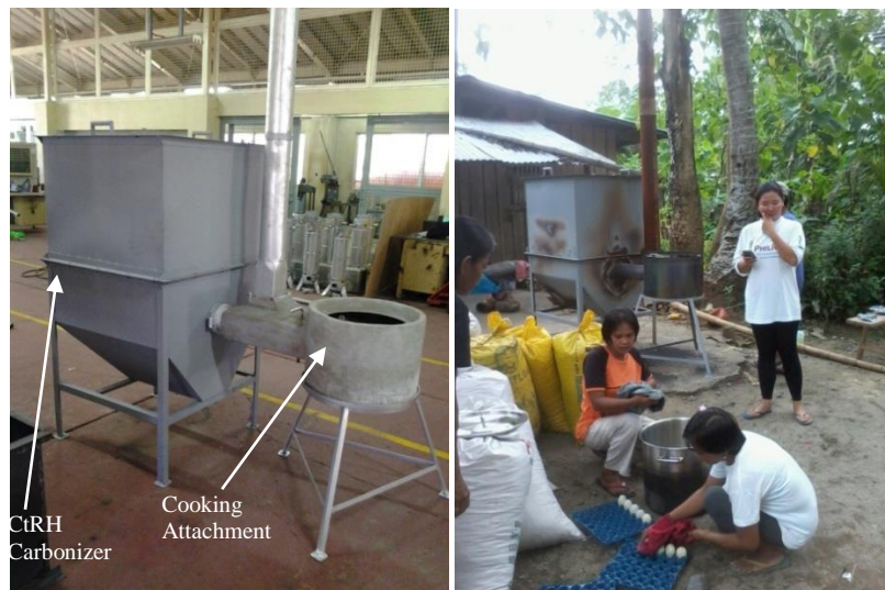
Figure 3. The carbonizer with the cooking attachment (left) and the cooked salted eggs (right).
