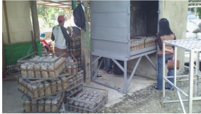
Figure 6. The 500-bag capacity mushroom pasteurizer coupled to the CtRH carbonizer.
