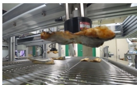
Image 2: Robot hand picking up a slice (Supplied by Iwate University)
