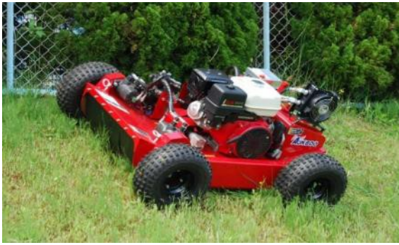
Remote-controlled mower working on a steep gradient
