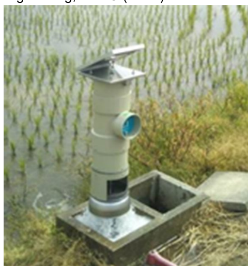
Fig.1 Sensor-equipped controller installed in a paddy (Provided by the Institute for Rural Engineering, NARO [NIRE])
