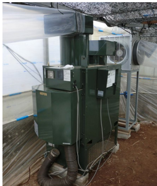
Fig.1 Carbon dioxide generator (Provided by the Kochi Agricultural Research Center)
