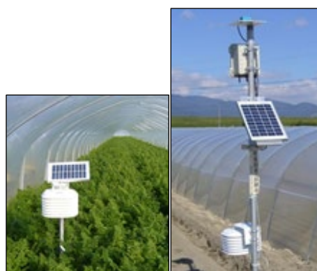
Fig.4 Installation status of the ICT environmental information system (left: temperature inside the greenhouse; right: outside temperature, etc.; provided by the Tokushima Agriculture, Forestry and Fisheries Technology Support Center)
