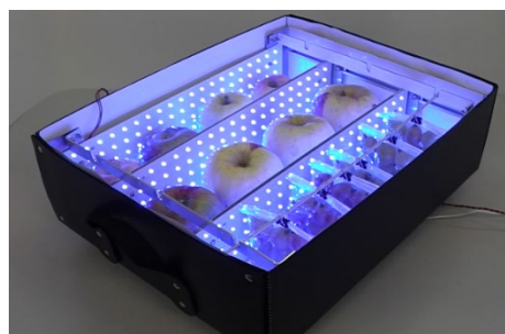
Fig.1 "Fruit coloration promotion device" that emits pale light (Provided by Yamaguchi Prefectural Industrial Technology Institute)
