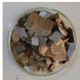
Fig.1 Semi-carbonized wood chips that have turned black (Provided by the Nara Forest Research Institute)
