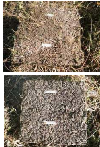
Fig.2 Conventional wooden pavement material (upper row) Developed product using semi-carbonized chips (lower row) (Provided by the Nara Forest Research Institute)
