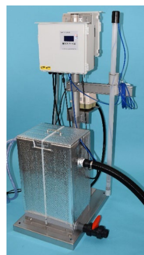
Fig.1 BOD monitoring system using electricity-producing bacteria (Provided by DKK-TOA Yamagata Corporation)
