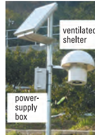
An automated air temperature data acquisition system
