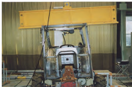
Rollover Protective Structure (ROPS) Test (Cush Test)
