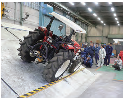
Measurement of static overturning angle of the tractor
