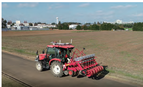
Automatically starts driving on farm roads after completing work in the field
