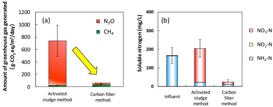
Fig. 6. Gas emissions and water quality in the activated sludge and carbon fiber bioreactors. (a) Amount of greenhouse gas generated from the bioreactors. (b) Water quality in the bioreactors.
