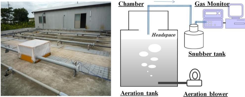
Fig. 3. System for measuring greenhouse gases from wastewater treatment plants.
