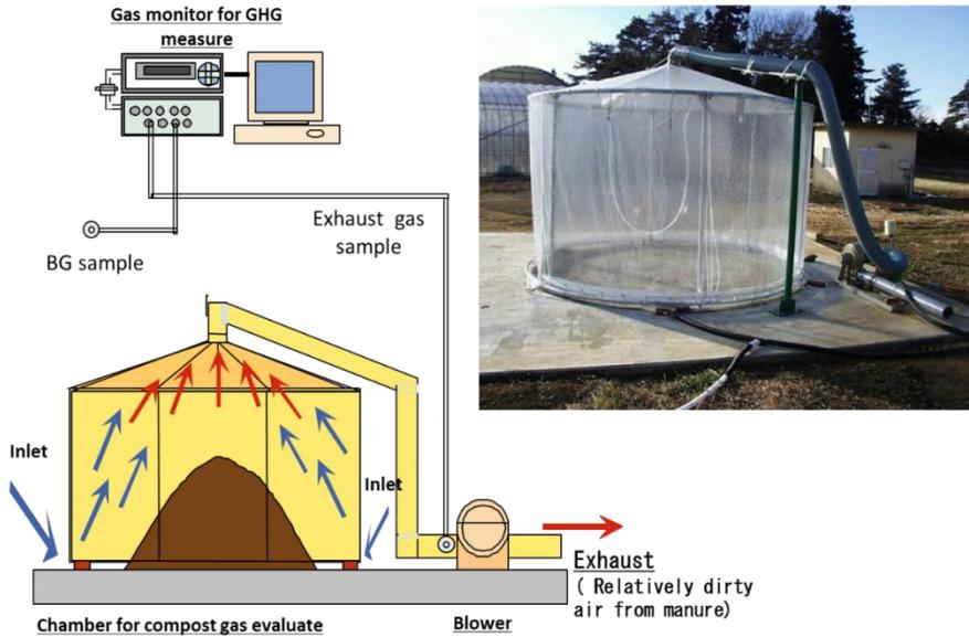
Fig. 1. System for measuring greenhouse gases from composting.
