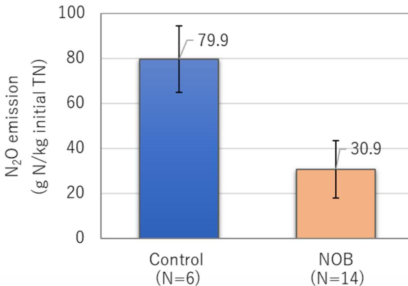
Fig. 4. Effect of NOB addition on N<sub>2</sub>O emission in laboratory-scale swine-manure composting experiments. Error bars indicate standard deviation.
