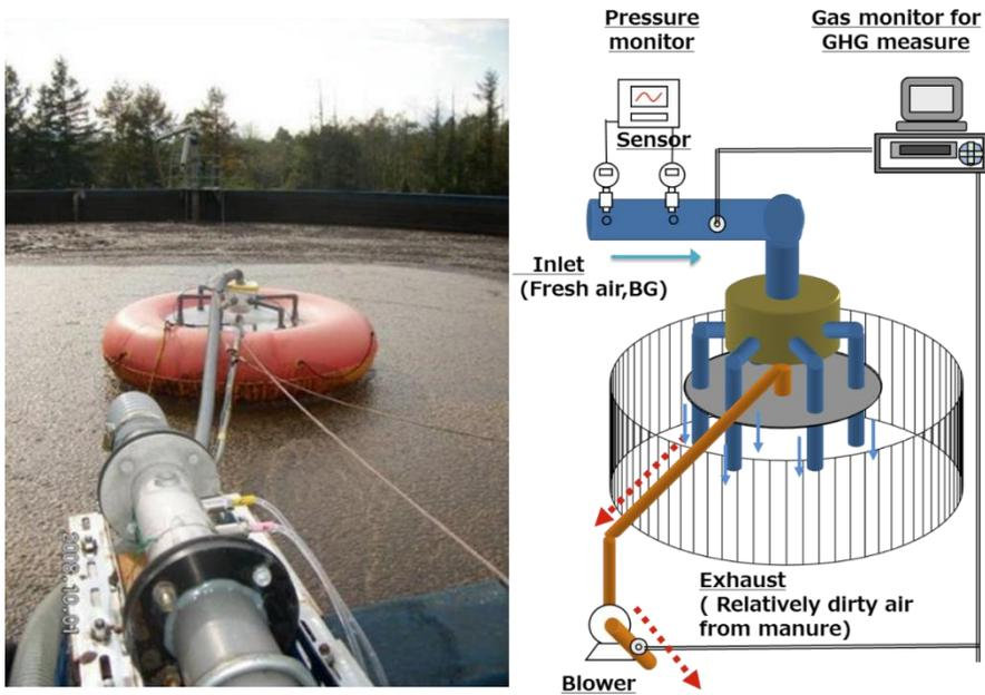
Fig. 2. System for measuring greenhouse gases from slurry storage.
