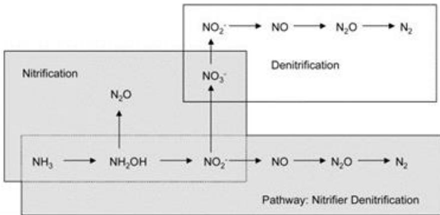
Fig. 5. Transformations of mineralized nitrogen (Wrage *et al.*, 2001).
