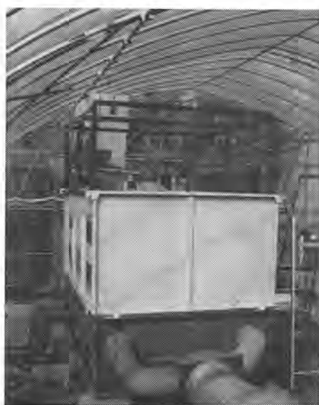
図31 静置式乾燥試験装置(実験2) Fig.31 Experimental stationary flat bed type air forced drier (Exp.2)
