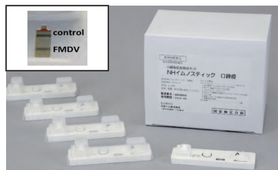
Silver amplification immunochromatography testing (ICT) kit for foot-and-mouth disease virus detection
