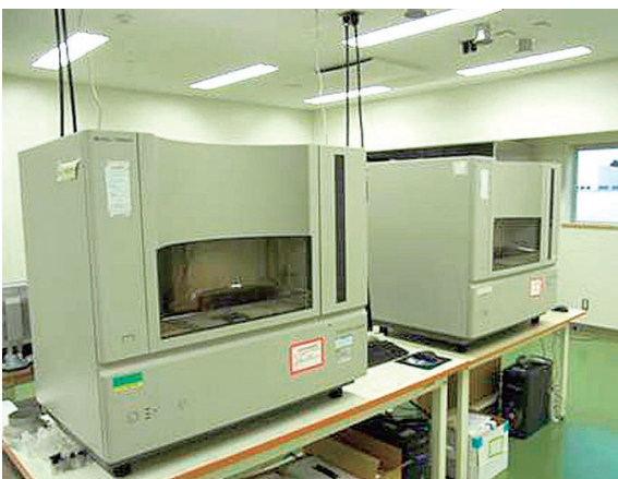
Fig. 3. Sanger sequencer (5 machines) We use these machines to determine valuable sequences for gene isolation and to detect the SNPs (Single Nucleotide Polymorphism) through DNA fragment analysis.
