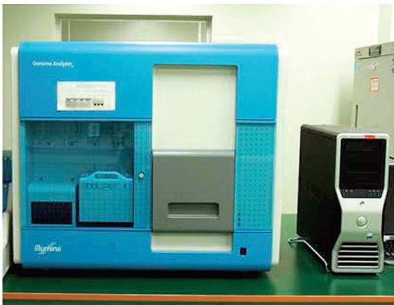
Fig. 1. Short read type sequencer (1 machine) We obtain about 40 giga (=40 billion) bases each run.
