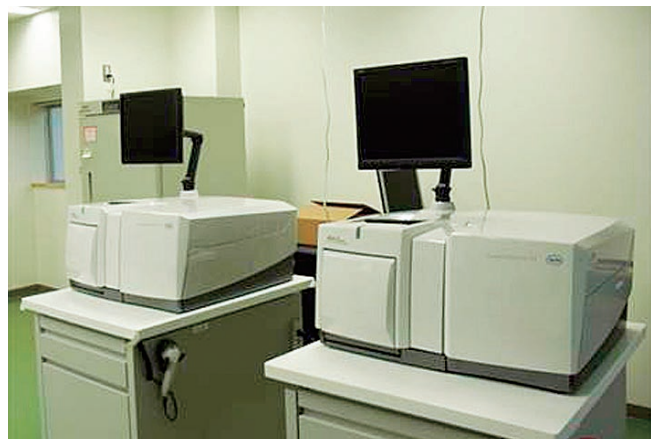
Fig. 2. Long read type sequencer (2 machines) Each machine produces 500 mega (=500 million) bases each run.
