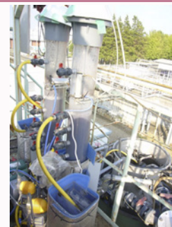
Mitigation of greenhouse gas emission from swine wastewater treatment in an aerobic bioreactor packed with carbon fibers.
