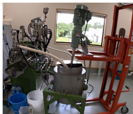
Photo 2: Wet-type bead milling process machine (photographed by Bio-oriented Technology Research Advancement Institution)
