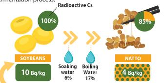
If soybeans with 10 Bq/kg radioactive Cs are processed into natto, the final radioactive Cs concentration is reduced to 4 Bq/kg.
