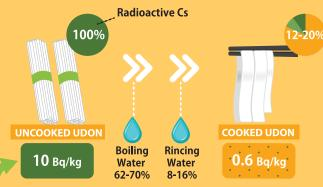
10 Bq/kg radioactive Cs in raw udon noodles is reduced to 0.6 Bq/kg radioactive Cs after boiling.
