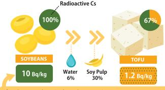
If soybeans with 10 Bq/kg radioactive Cs concentration are processed into filling tofu, the final radioactive Cs concentration will be 1.2 Bq/kg.
