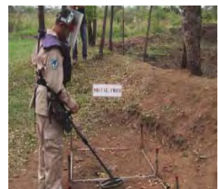
Calibration of Metal Detector before task (Thailand)
