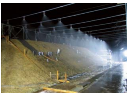
■ Rainfall test on a full-scale reservoir
