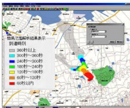
■ Predicting the flood area due to bank failure
