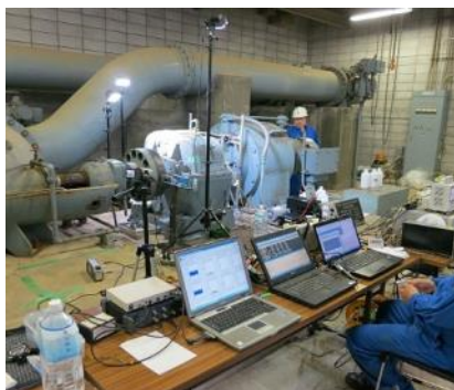
■ Deterioration promotion test of pump facilities
