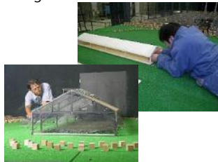
■ Large-scale wind tunnel testing for agricultural structure and environment
