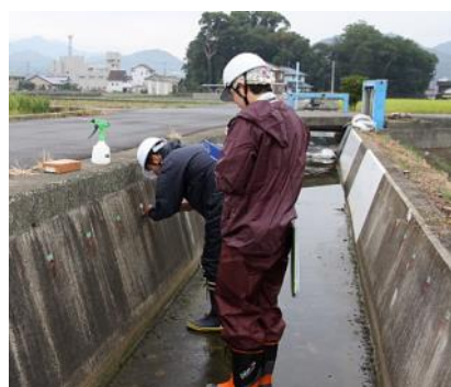
■ Field survey of repair material long-term durability
