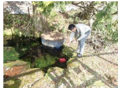
■ Water sampling from a spring-fed pond to measure environmental isotopes
