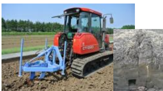
New subsoil breaker which inserts no drainage material: "Cut Drain" (characterized by deep breaking and long-lasting drainage voids)
