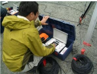
■ Using a new exploratory method to check the distribution of available groundwater
