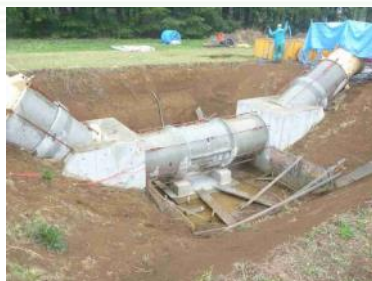
■ Liner pipe experiment with full-size model
