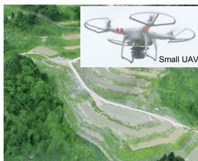
■ 3D modeling of terraced paddy fields based on UAV aerial photo images
