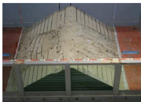
■ Experiment to verify the destruction mechanism of earthquakes
