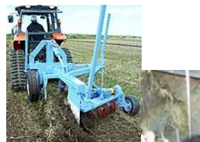
New subsoil breaker that inserts drainage material: "Cut Soiler" (forms drainage channels in the soil that are filled with crop residue and other materials from the surface)
