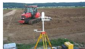
Labor-saving and precise field management technologies using highly accurate GPS (leveling requires about 40% less labor than before)
