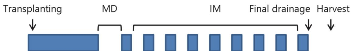
**Figure 2.2.** Typical practice of paddy water management in Japan. Midseason drainage (MD) at the rice-tillering stage for a period of 5–7 days is followed by intermittent irrigation (IM) that involves repeated periods of alternate flooding and drying, each for a few days.
