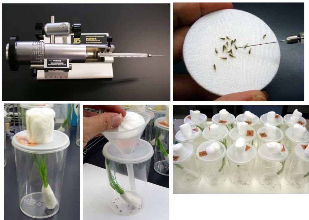
Fig. 16. The standard method: a hand micro-applicator.
