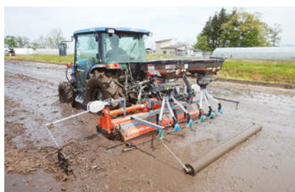
Direct seeding of uncoated rice seeds in shallow soil by paddy harrow seeder
