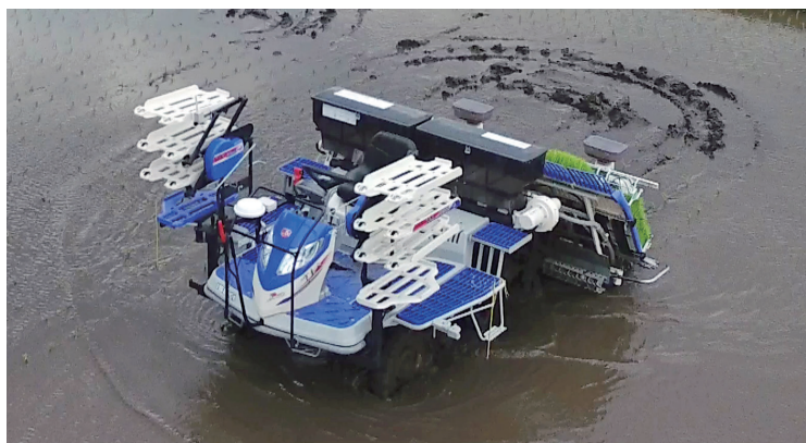
Autopilot rice transplanter developed by NARO through a national project "Cross-ministerial Strategic Innovation Promotion Program (SIP)" and is ready to go to market in February 2022
