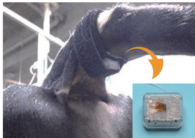
Body temperature sensor attached to the ventral tail base.
