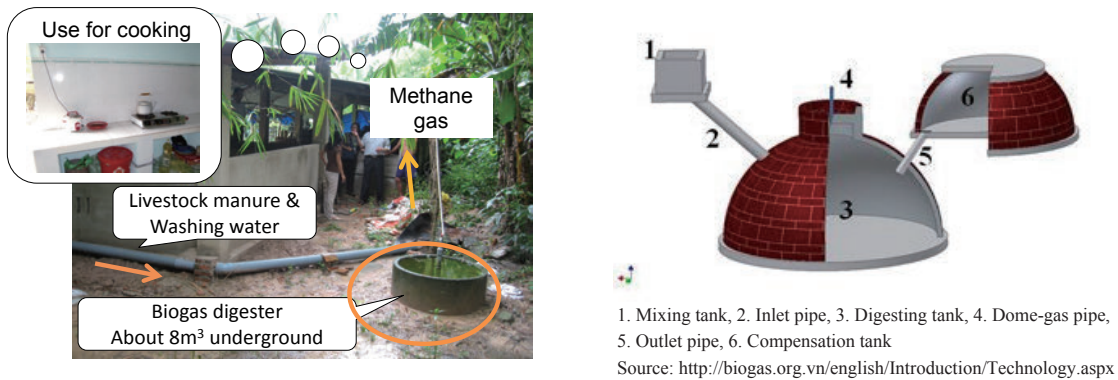
Fig. 1 Fixed dome type of household biogas digester
