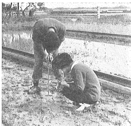
第 I - 6 図 矩形板沈下量測定状況 (Fig. I-6. Measuring the sinkage of rectangular plate)
