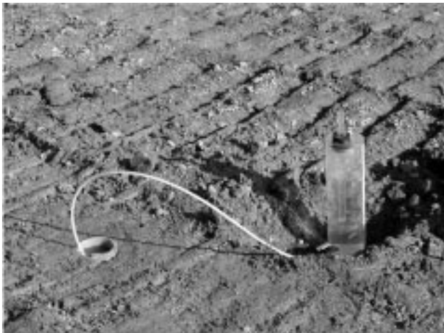
Photo 7 一定水位型現場透水試験器 Example of field permeability test apparatus
