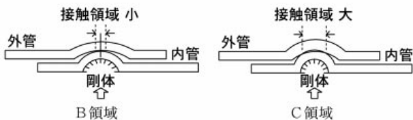
Fig.19 FEM解析による内管と外管間に作用する応力 Stress to act between inside pipe and the outside pipe by F.E.M.analysis
