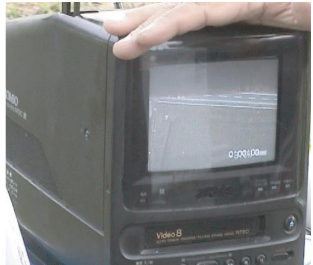
Fig.5 地上モニターによる撮影範囲の確認 Confirmation of the taking area used by a monitor on the ground
