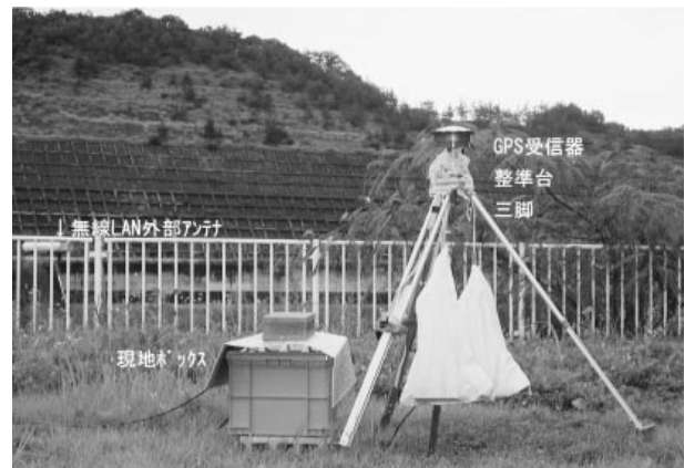
Fig.7 GPS基準点状況 Situation of GPS datum point
