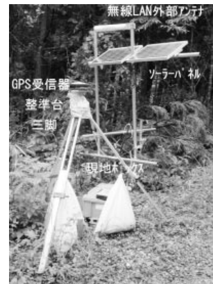
Fig.6 GPS移動点状況 Situation of GPS monitoring point
