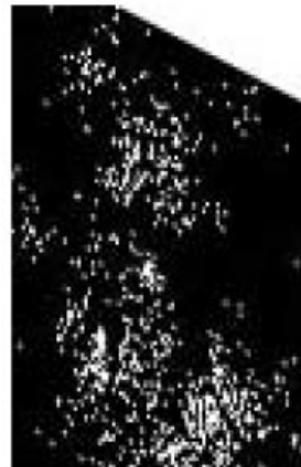
Fig.14 8-近傍オープン操作 (収縮処理後に2回膨張処理)(閾値=1800以下) 8-neighbour opening after erosion double dilation (threshold=under 1800)
