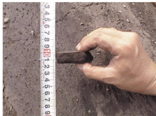
Date: 2005/9/22 Fig.12 土壌表面に形成した硬い土壌層 (CT) Hard soil layer formed on soil surface (CT)
