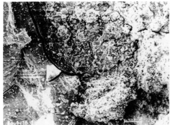
Fig.8 飛沫部コアの白色析出物SEM画像 SEM picture of white separating in splash area
