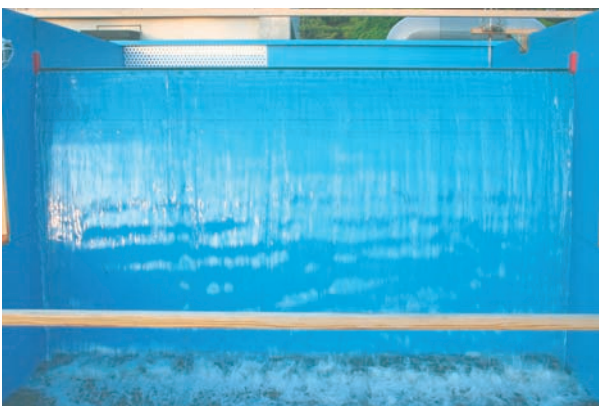
Fig.14 スポイラ間隔3mの場合の越流水膜 (越流水深0.03m) Falling water sheet for spoiler interval 3m (overflow depth 0.03m)
