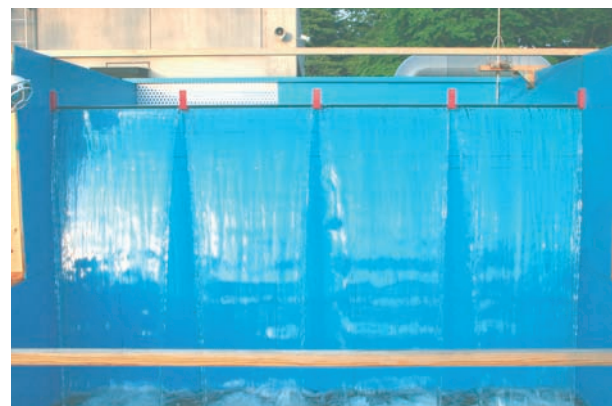
Fig.17 スポイラ間隔0.75mの場合の越流水膜 (越流水深0.03m) Falling water sheet for spoiler interval 0.75m (overflow depth 0.03m)
