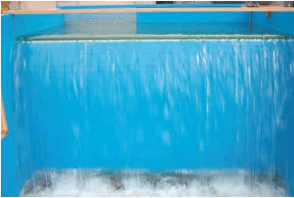
Fig.13 スポイラなしの場合の越流水膜 (越流水深0.03m) Falling water sheet for no spoilers (overflow depth 0.03m)
