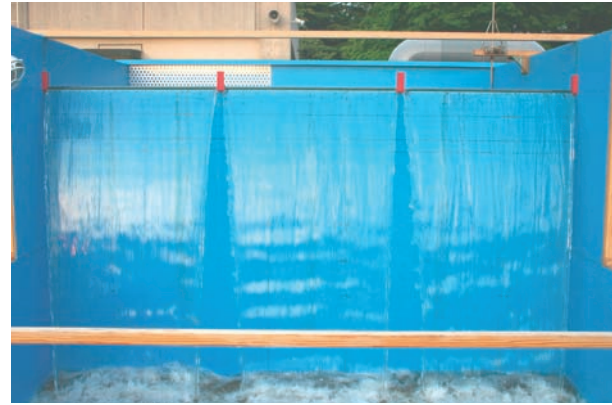
Fig.16 スポイラ間隔1mの場合の越流水膜 (越流水深0.03m) Falling water sheet for spoiler interval 1m (overflow depth 0.03m)
