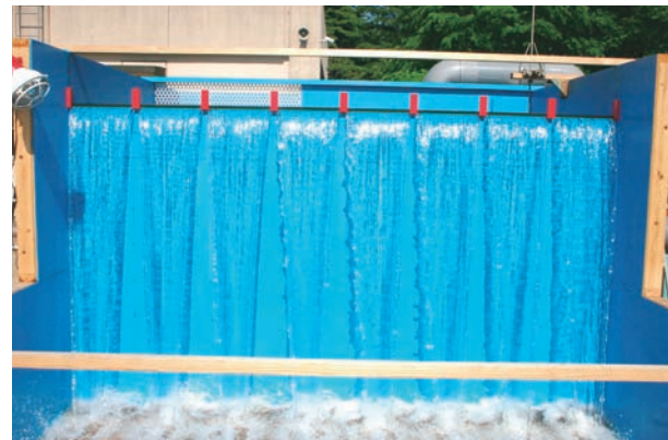
Fig.18 スポイラ間隔0.375mの場合の越流水膜 (越流水深0.03m) Falling water sheet for spoiler interval 0.375m (overflow depth 0.03m)
