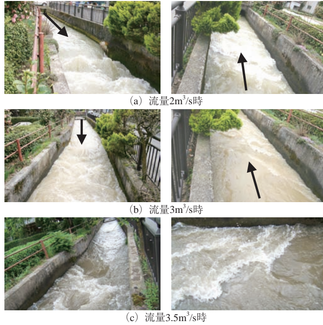
Fig.7 Y号落差工位置の流況 Flow at Yth ground sill
