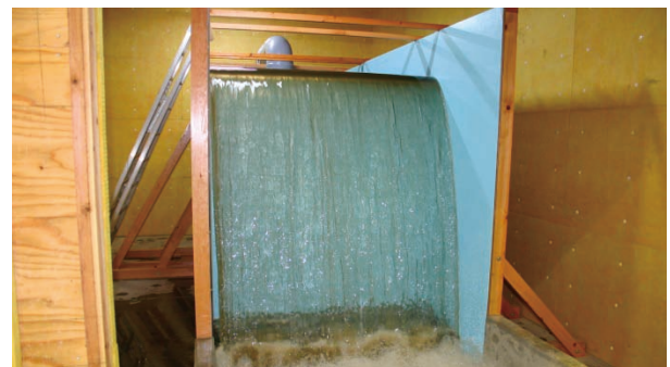
Fig.2 越流堰の水理模型 Hydraulic model of overflow weir
