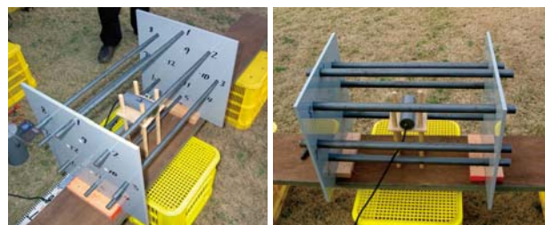
Fig. 16 主鉄筋影響試験 (鉄筋径 φ 13, φ 25, L = 50cm) View of effect test for reinforcing bar (diameter φ 13, 25mm, length = 50cm)
