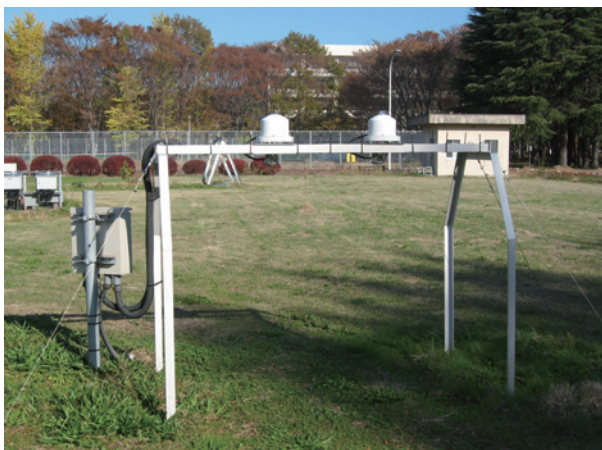
Fig.6 短波・長波放射量観測の状況 Observation of short- and long-wave radiations
