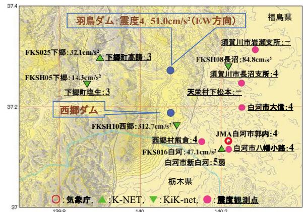
Fig. 28 羽鳥ダムと西郷ダムの近傍の強震観測点（JMA, K-NET, KiK-net）の震度と最大加速度 Seismic intensity and maximum acceleration of strong motion stations near Hatori dam and Nishigou dam
