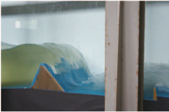
Fig. 7 海岸堤防の越流状況 Photo of tsunami overflows the coastal dike
