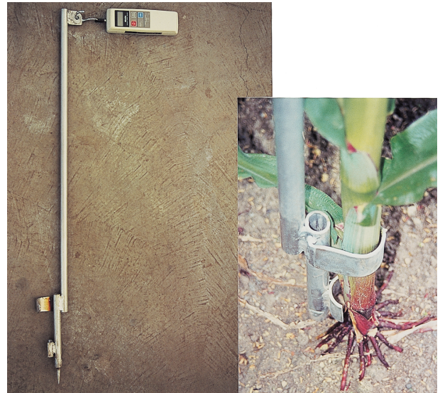
Photo 2. Aluminum stick and digital force gauge used for measurement of horizontal pulling resistance (left) and the stick attached to base of the stalk (right)
