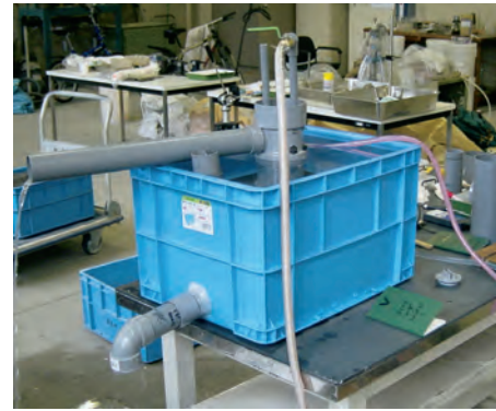
Fig.4 透水試験装置の外観 Outward appearance of a permeability test apparatus.
