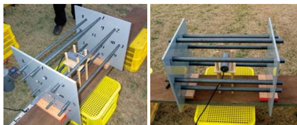
Fig. 16 主鉄筋影響試験 (鉄筋径 φ 13, φ 25, L = 50cm) View of effect test for reinforcing bar (diameter φ 13, 25mm, length = 50cm)
