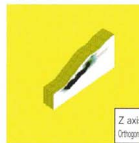
■ Maximum shearing distortion at the time of collapse (three-dimensional analysis of a landslide)
