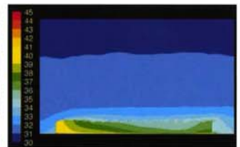
■ CFD analysis of greenhouse temperature distribution in the summer
