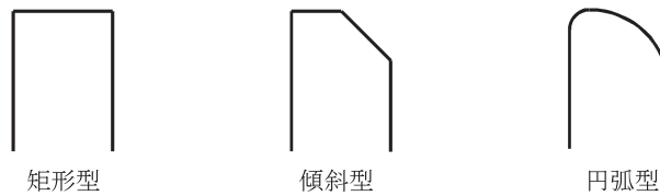
Fig. 2 階段式魚道の隔壁天端の縦断面図(左が上流) Side view of the crown of the weir wall in pool-and-weir type fishway (from the right side)
