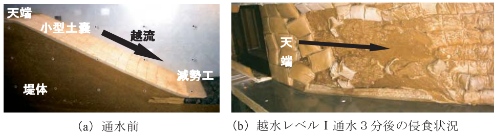
Fig. 218 Case01 (小型土嚢を堤体斜面に敷き並べたタイプ)の観察結果 Observation of Case 01 (surface protected with small soil bags arranged along the slope surface)
