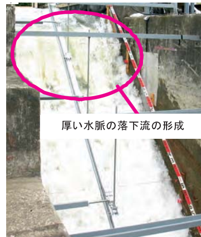
Fig. 235 Skimming flow 時の堤体下流斜面の流況 ( q = 0.348 \text{ m}^3/\text{s/m} ) Stream regime on downstream slope at skimming flow
