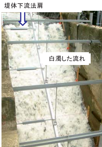
Fig. 234 Nappe flow 時の堤体下流斜面の流況 ( q = 0.087 \text{ m}^3/\text{s/m} ) Stream regime on downstream slope at nappe flow
